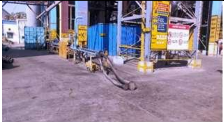
Pneumatic System available for unloading and feeding of Carbon black powder to the mill
